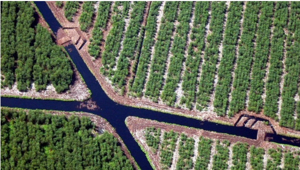
Figure 2: Canal system in pulp wood plantation on 5-10 m deep peat in Kampar region. Note the dams with the by-passes.
