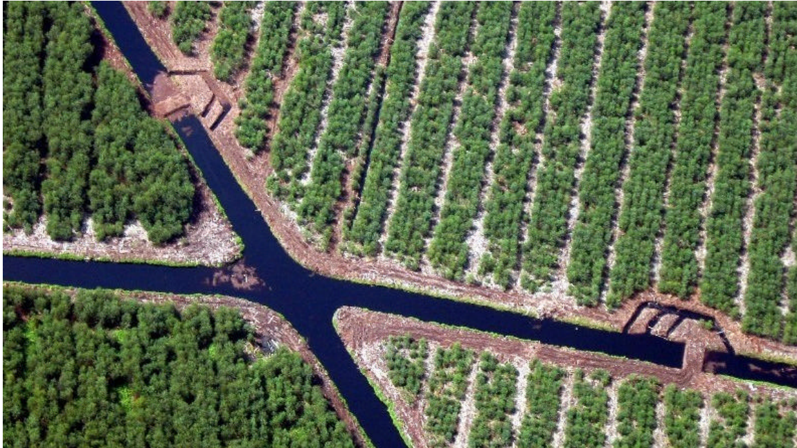
Figure 2: Canal system in pulp wood plantation on 5-10 m deep peat in Kampar region. Note the dams with the by-passes.
